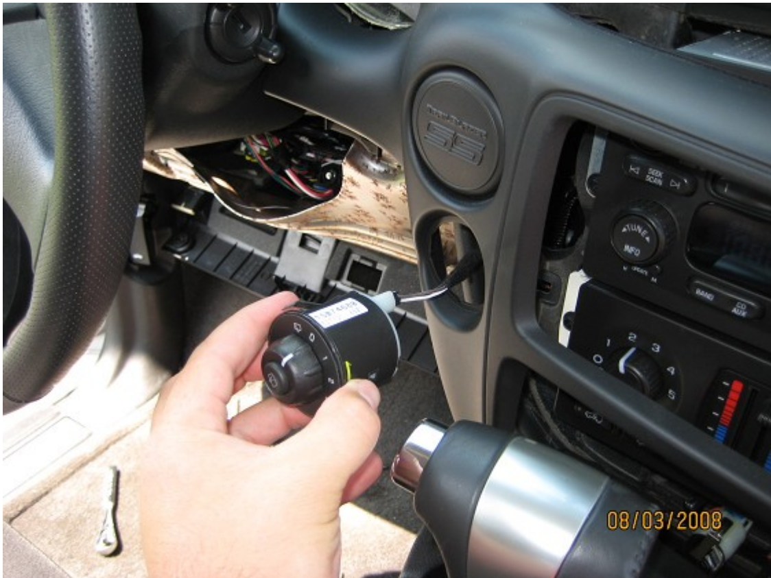
13. The TBSS plug pops out the same way (no connection though)
