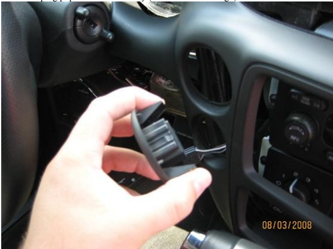
13. The TBSS plug pops out the same way (no connection though)
