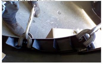
6) Apply a faster curing adhesive (10+ minutes) to the tab area insuring adhesive penetrates holes and covers bumper tabs
