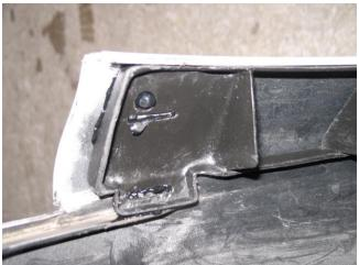
5) If necessary, at adhesive contact points, apply pressure against clip and bumper or clamp to thin adhesive and insure a flush fit against the bumper. **NOTE**: Insure that clip is within previously drawn outline before adhesive fully cures. **Flush fitment of clip against bumper is critical for proper bumper fitment**.
