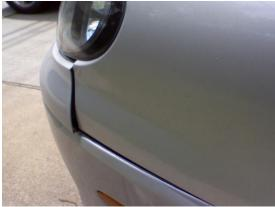
NOTE: The repair and replacement of the front bumper clips should ONLY be performed by an auto body professional. General Motors did not intend for OEM bumper clips (3) be replaced. OEM clips have a small opening at the end of the clip attachment section as it mate with the body mount clip (5). Ours does not and is a solid piece with an indentation. Therefore, it may be necessary to trim away extra material from this indentation area to insure a flush and secure fit.
